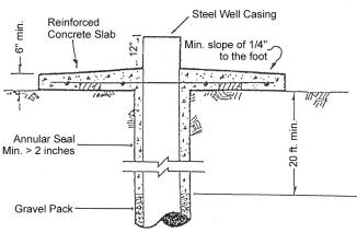
**Dimensions:** The slab must extend horizontally at least three feet from the center of the well casing in all directions.
